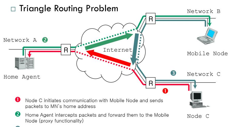
3 Mobile Node replies directly to Node C
