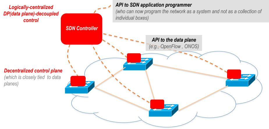
At the highest level, the SDN movement is an effort to build networks you can program at a higher level of abstraction— just as you can program a computer.
