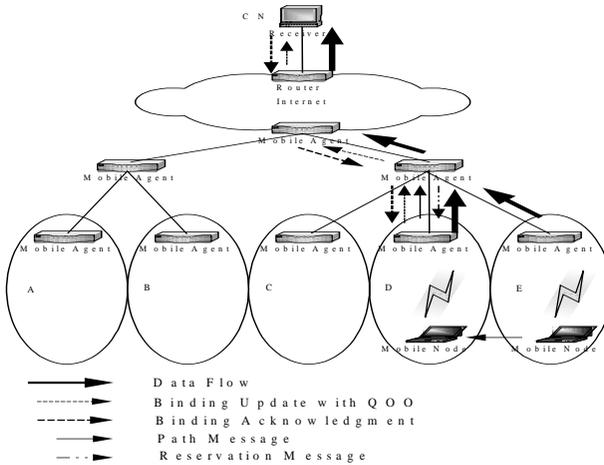
Fig. 2. MN as Sender in HMAT Model
