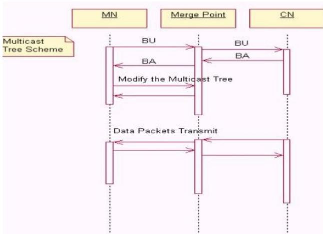
Fig. 4. Sequence Diagram of the Multicast Tree Scheme
