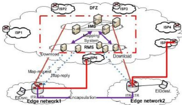
Fig5. Packet forwarding using HMS
