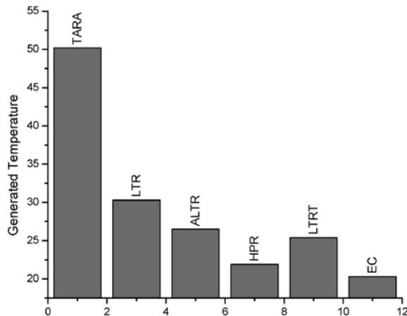
Figure 1: Performance comparison of event based communication (EC) with TARA, LTR, ALTR, HPR and LTRT. EC generates less amount of temperature than other protocols. TARA generates the maximum temperature, ALTR is better than LTR for the use of hop count threshold. HPR is better than LTR, ALTR or LTRT but EC provides the least temperature.
