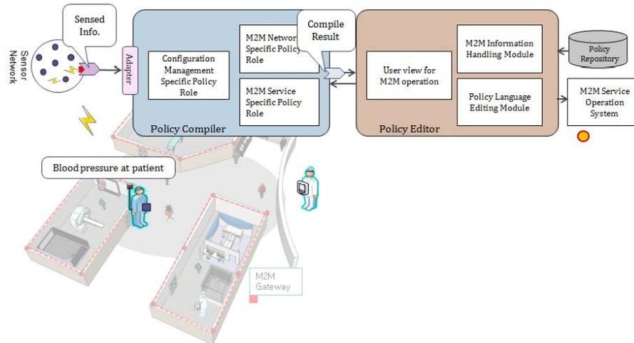
Figure 6: Implementation scenario of proposed system. Temperature is sensed by remote patient and specific policy rule is executed to send notification information to remote doctor in a ubiquitous health monitoring environment
