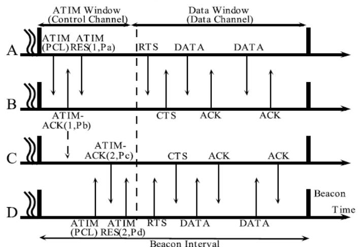
Fig. 2. Negotiation and data exchange in MMAC-PC
