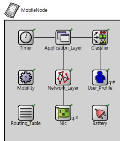
Figure 4. Implemented Mobile Device for Simulation
