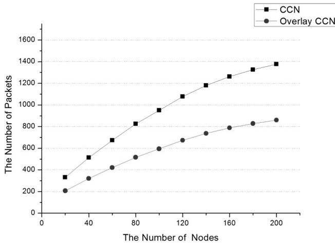
Figure 6. Comparing increasing the number of packets as the number of nodes for finding content
