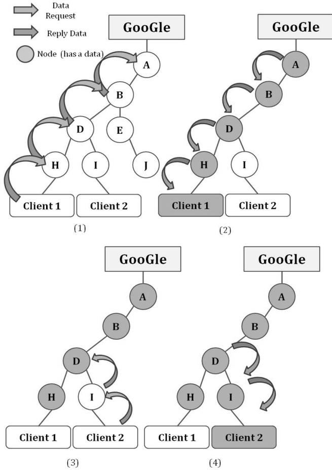
Figure 1. Basic Routing Scheme for CCN
