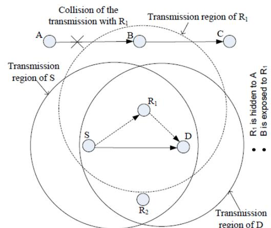
Fig. 1 Retransmission of  $R_1$  enlarging the transmission region: hidden and exposed terminal problem appears
