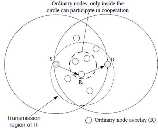
Fig. 2 Network model: transmission of R does not enlarge the transmission region of S and D
