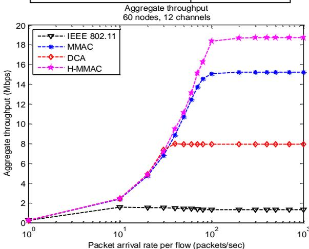
Fig. 2. The throughput of different protocols.
