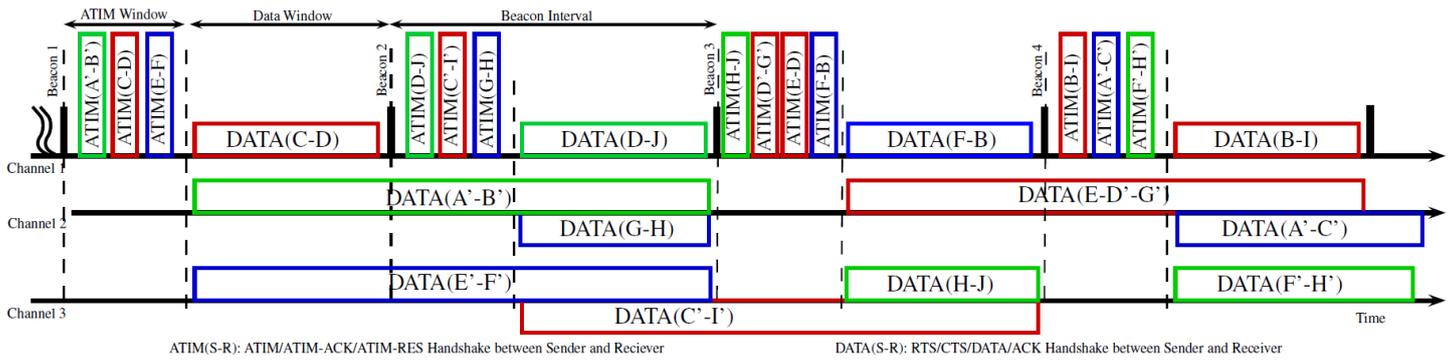
Fig. 1. The operation of H-MMAC protocol.
