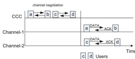
Fig. 1. Process of channel negotiation and data communication with a common control channel
