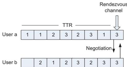
Fig. 2. Operation of a channel hopping protocol
