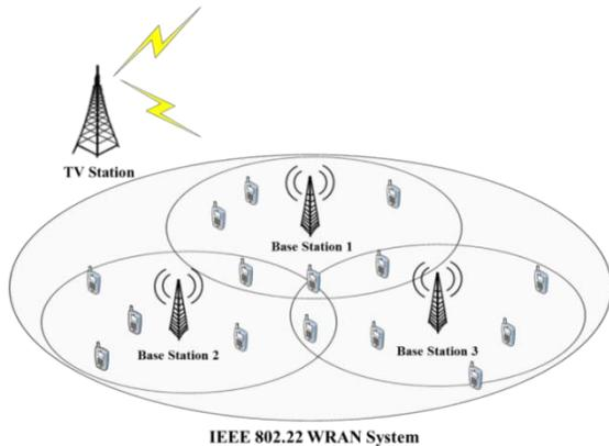
Figure 4 Deployment of IEEE 802.22 WRAN System
