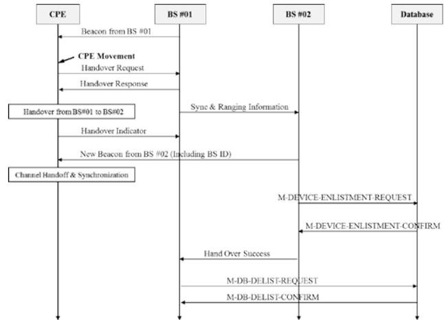
Figure 7 Handover Procedure of IEEE 802.22 WRAN
