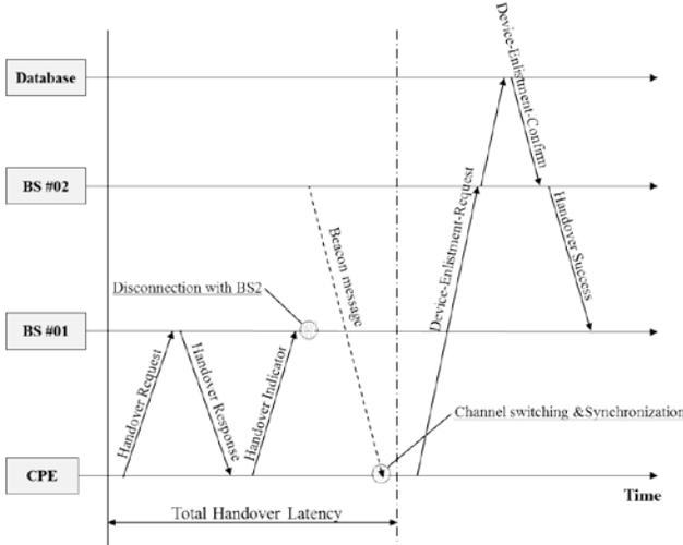
Figure 13 Handover latency of proposed mechanism
