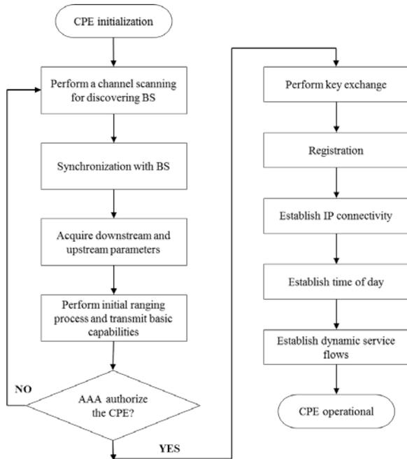
Figure 1 The procedure of CPE initialization
