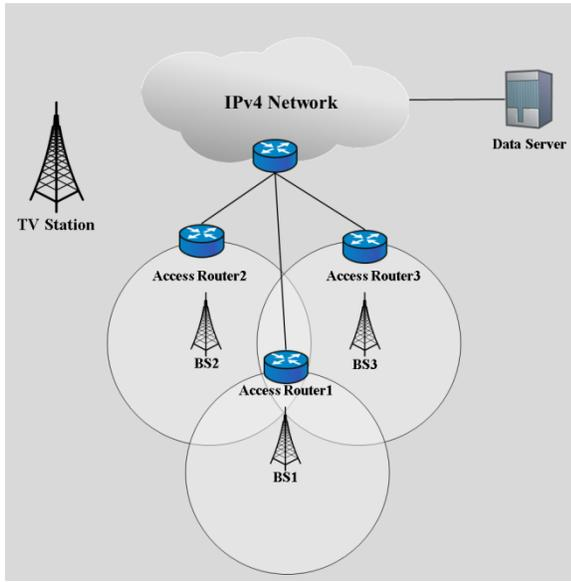
**Figure 12 Simulation model of IEEE 802.22 WRAN system**
