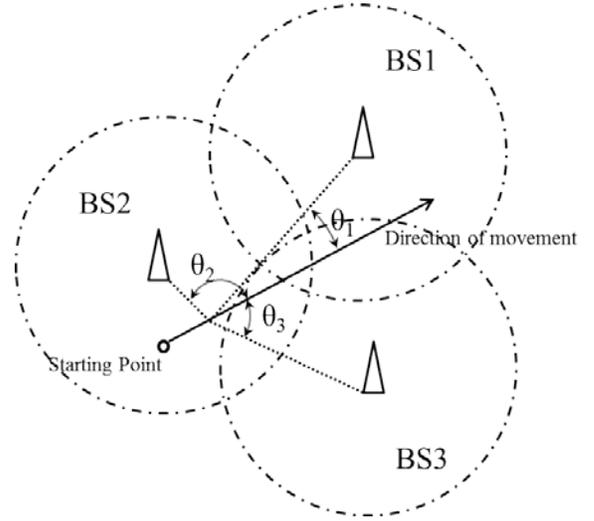
**Figure 10 Algorithm for selecting Target BS**
