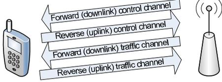
**Figure 3: Uplink and downlink channels**
