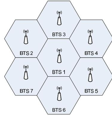
Figure 1: 7-Cell Configuration
