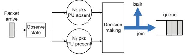
Fig. 2. Hybrid overlay/underlay decision making.
