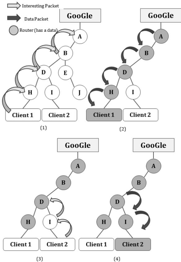
Figure 2. Basic Routing Scheme for CCN
