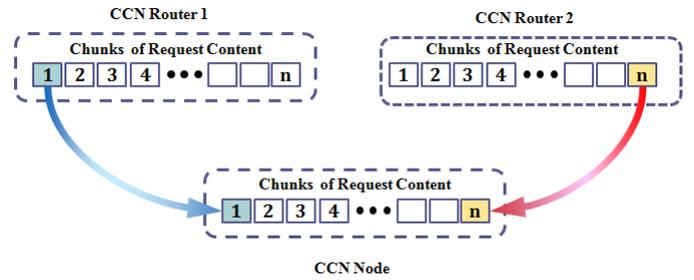
Figure 6. Bi-Directional Content Delivery using the last number of chunk
