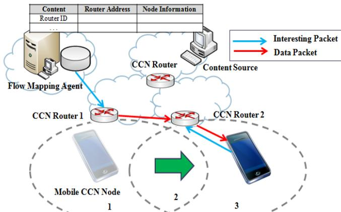
Figure 4. Architecture of CCN using flow mobility
