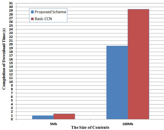
Figure 9. Comparing Completion of Download Time between Proposed Scheme and basic CCN
