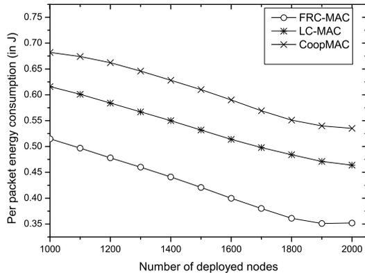
Fig. 10. Energy efficiency vs. number of deployed nodes for different protocols
