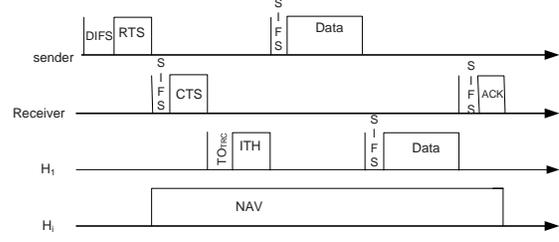
Fig. 4. Frame sequence for TRC mode
