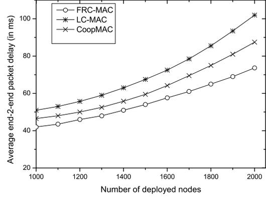
Fig. 9. end-to-end delay vs. number of deployed nodes for different protocols
