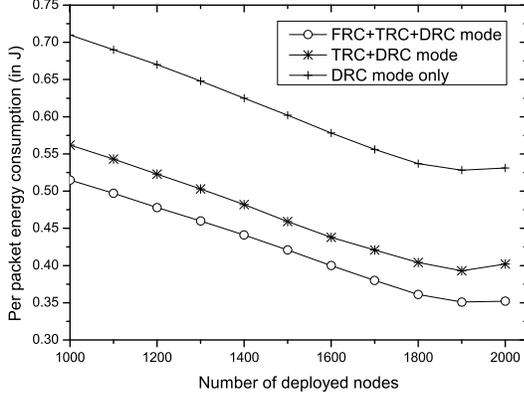
Fig. 7. Energy consumption vs. number of deployed nodes for different communication modes
