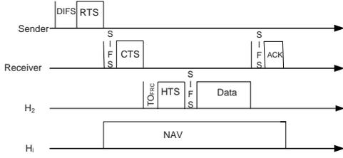
Fig. 5. Frame sequence for FRC mode
