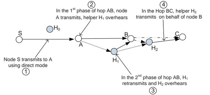
Fig. 1. Basic network model: DRC, TRC and FRC modes are used in the hop  $SA$ ,  $AB$  and  $BC$  respectively
