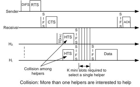
Fig. 6. Frame sequence for FRC mode when collision occurs
