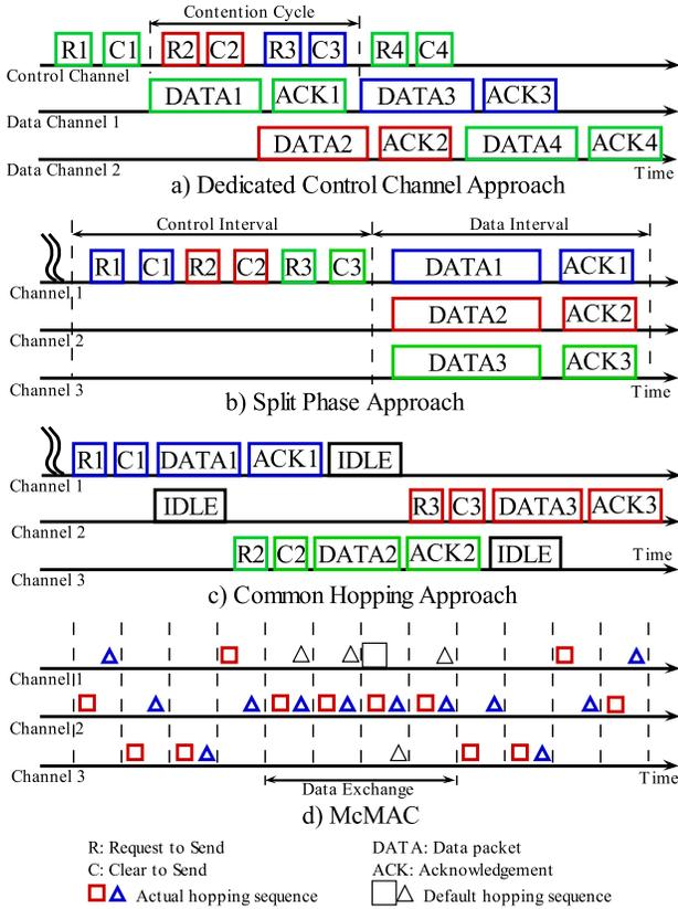
Fig. 1. Four approaches for multi-channel MAC protocol.[2]
