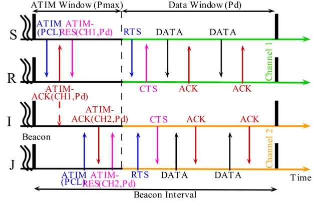
Fig. 3. The operation of E-MMAC protocol.
