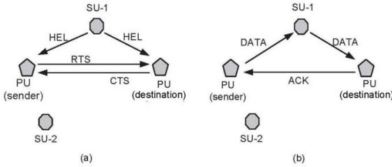
Fig. 2. (a) Control packets exchanges between PUs and the helper (SU), and (b) cooperative data transmission.
