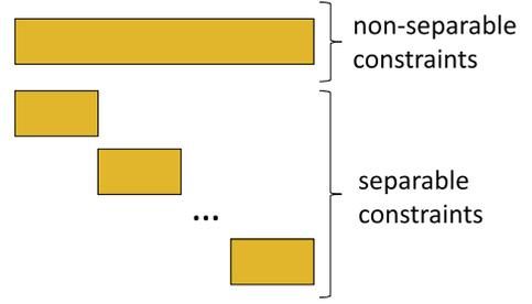
**Fig. 2.** The block-angular structure of the primal problem.
