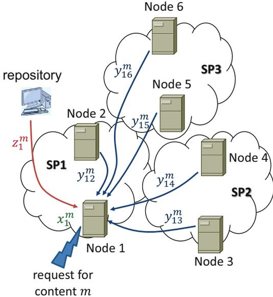
**Fig. 1.** Example of cooperative caching in a content-oriented network with three SPs. Node 1 receives  $y_{1i}^m$  fraction of content from node  $i$  and  $z_1^m$  fraction of content from  $m$ 's repository to serve the request for content  $m$  at node 1 containing  $x_1^m$  fraction of content.
