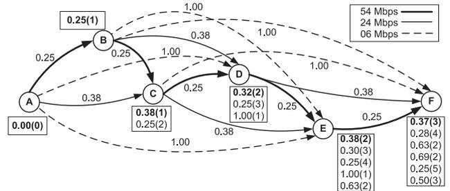
**Fig. 3** An example of using the path gain metric with 3 supported rates. All paths source at A and the link gains are taken from Table 1 (with RTS/CTS handshaking). The table at a node shows the available path gains with corresponding hop-count at the node.
