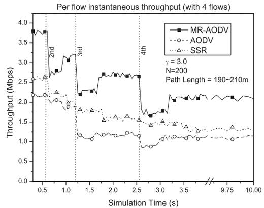
Fig. 7 Instantaneous end-to-end throughput with 4 flows. The flows start at 0.00 s, 0.60 s, 1.20 s and 2.60 s time instants. The route discovery phase for the first flow is not shown in the figure.
