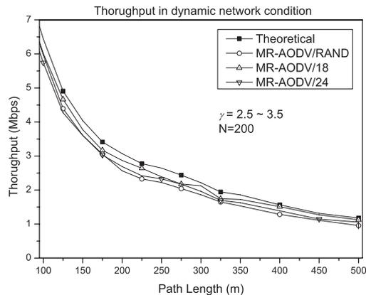
**Fig. 8** Throughput performance of MR-AODV in a stochastic environment.
