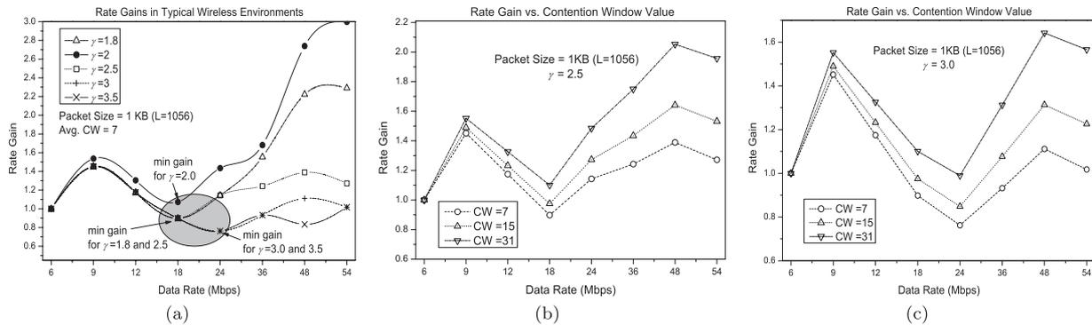
**Fig. 4** Rate Gain vs. attenuation factor ( $\gamma$ ) and contention window size (CW): (a) impact of  $\gamma$  (with CW=7), (b) impact of CW (with  $\gamma = 2.5$ ), and (c) impact of CW (with  $\gamma = 3.0$ ).
