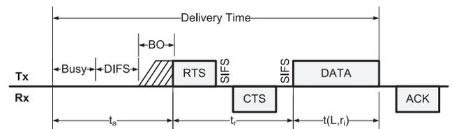
Fig. 1 Packet delivery time.
