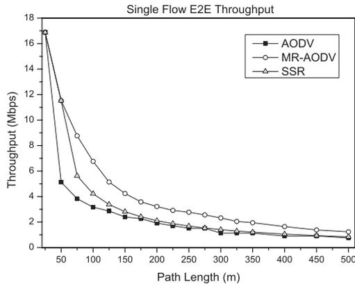
Fig. 6 End-to-End Throughput for single flow.
