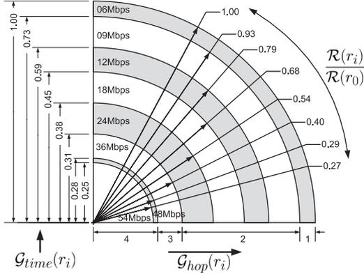
**Fig. 2** Hop and time gains for different rates in the IEEE 802.11g PHY ( $\gamma = 3.0$ ,  $t_a = 50 \mu s$ ,  $t_r = 0.128$  ms and  $L = 1056$ ).
