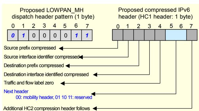
Fig. 3. Proposed LOWPAN\_MH dispatch header pattern and compressed IPv6 HC1 header.
