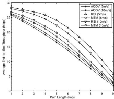
Fig. 4. Average Throughput Vs. Path Length.
