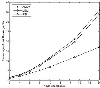
Fig. 2. Percentage of Broken Links Vs. Mobility.
