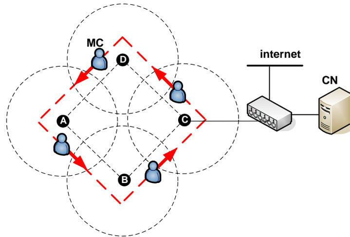
**Fig. 10.** The mesh network testbed topology.
