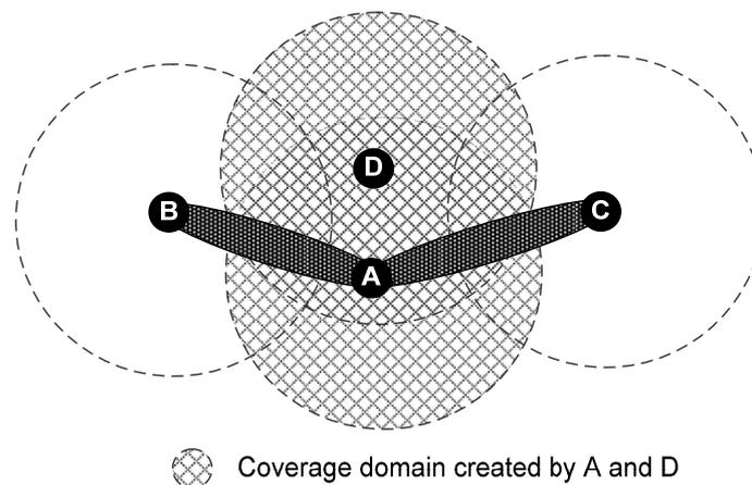
Fig. 2. Coverage-oriented configuration to expand coverage.
