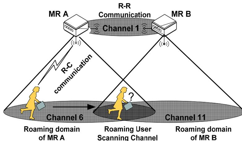
Fig. 1. A typical multi-radio multi-channel WMN.
