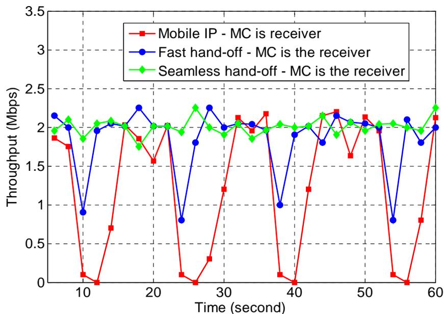
Fig. 13. TCP throughput observed at the CN node.
