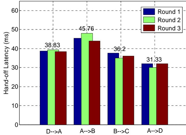
Fig. 11. Hand-off latencies for various pairs of mesh routers.
