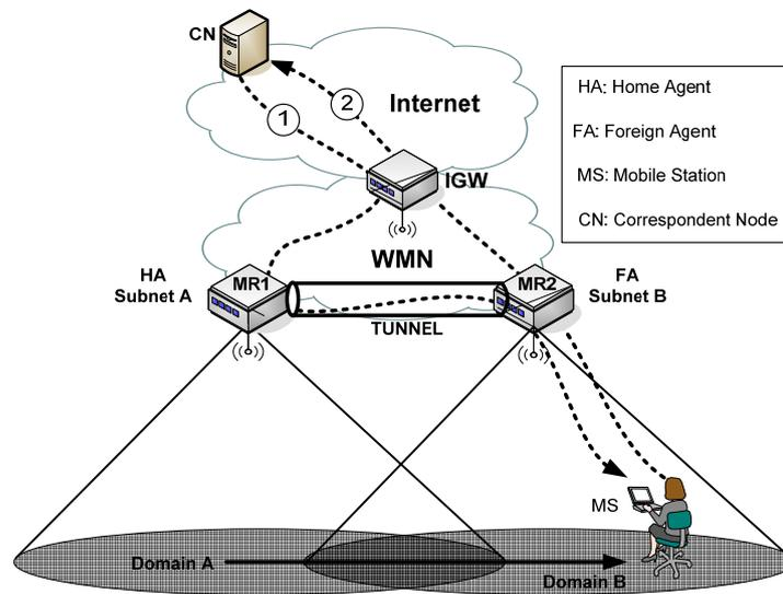
Fig. 5. Typical terms for the Layer-3 roaming process.
