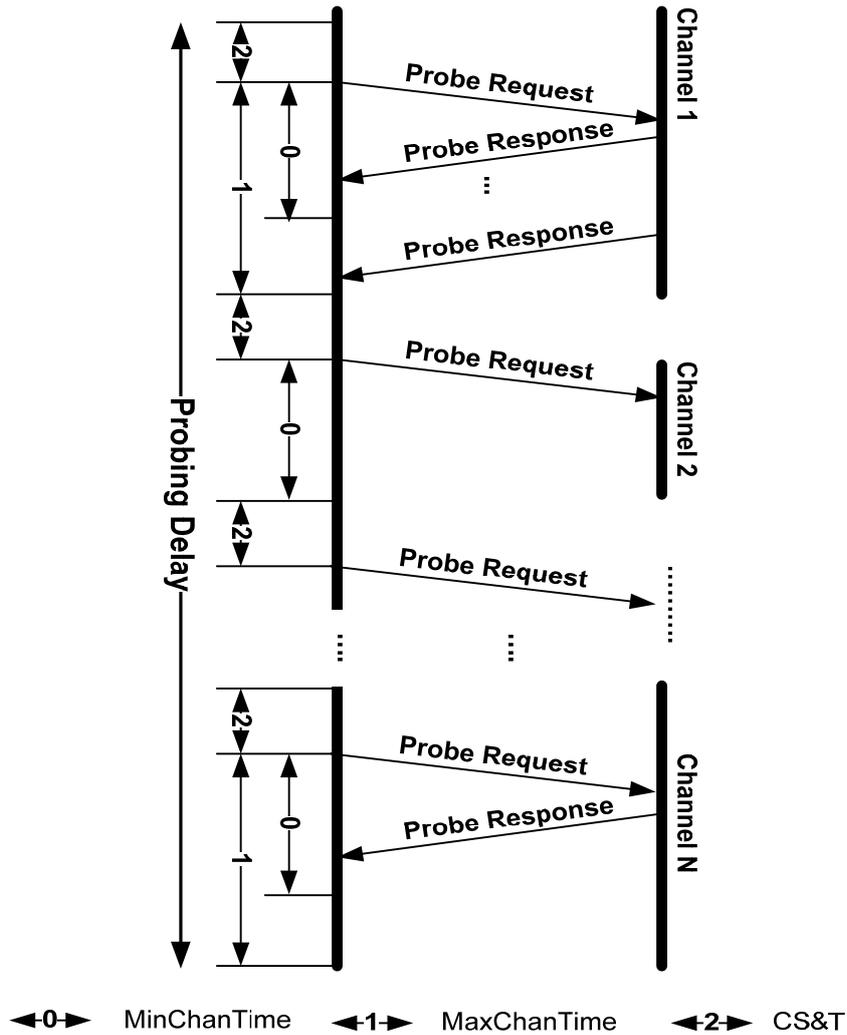
Fig. 4. The probing process in the IEEE Standard 802.11.
