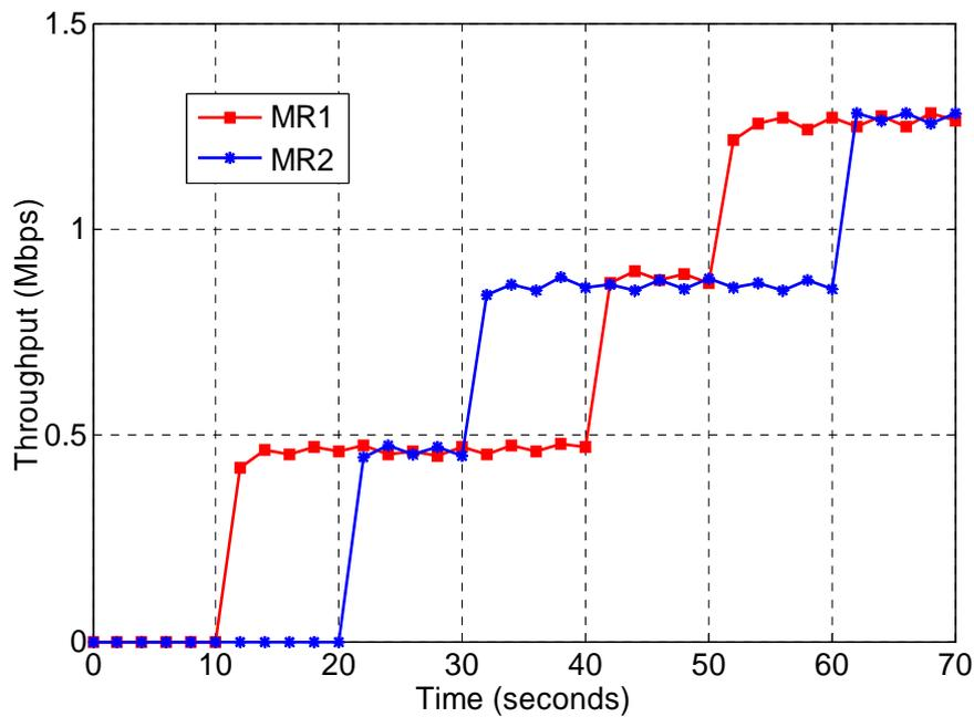
Fig. 15. Load-balancing between two MRs.
