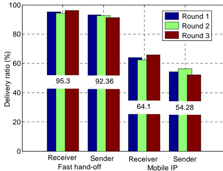
Fig. 12. PDRs seen at both the receiver and sender.
