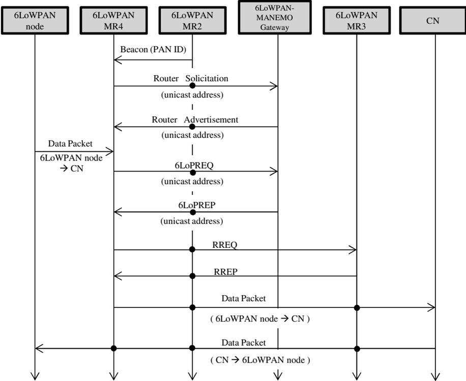
Fig. 4. Proposed signaling flow for supporting the optimal path in 6LoWPAN based MANEMO networks
