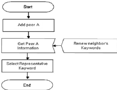
Figure 7. A flowchart of joining new peer
