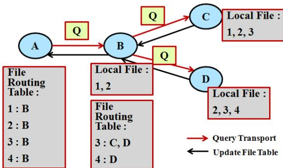
Figure 4. Searching resource using Optimized Routing Independent Overlay Network (ORION)
