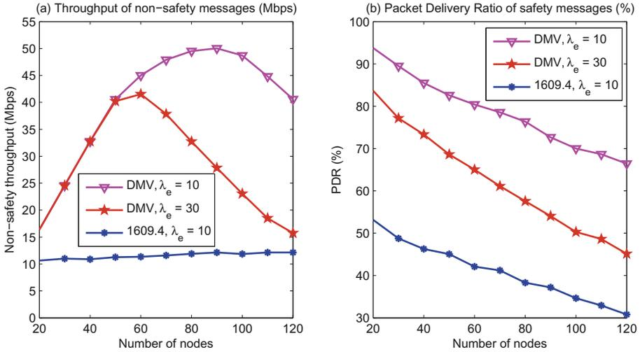
**Fig. 6.** Performance comparison of the IEEE 1609.4 and DMV protocols.
