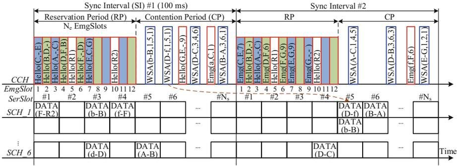
Fig. 5. The operation of the DMV protocol.
