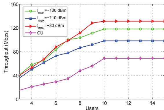
Figure 3: Average throughput under various tolerance levels.
