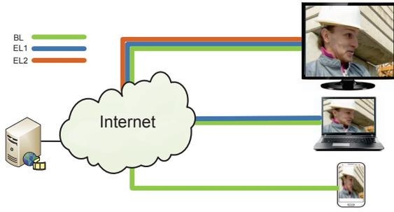
Fig. 1: H.264/SVC encoded video delivery to various devices with different device capabilities/bandwidth
