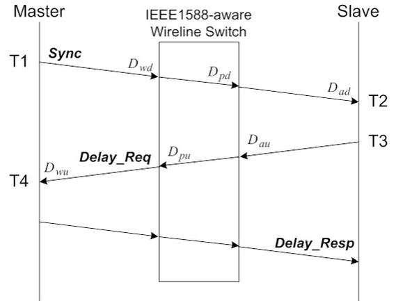
Fig. 1. IEEE 1588 messaging timing diagram.
