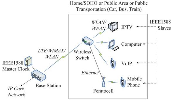
Fig. 2. IEEE 1588 PTP for wireless network.
