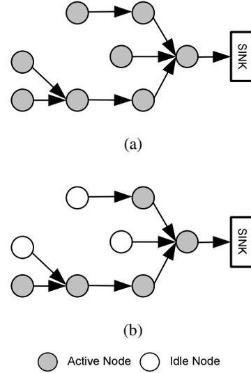
**Figure 4: Active and Idle Sensor Nodes Scenario**
