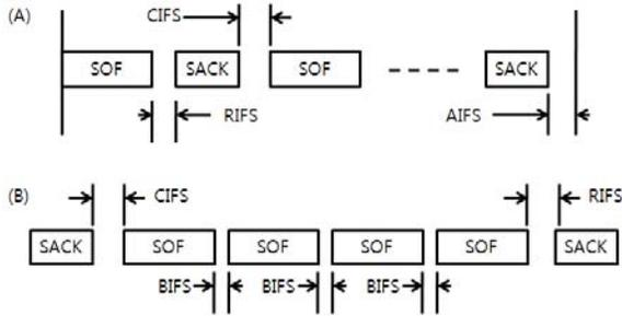
Figure 3. Inter-frame Spacing and MPDU Bursting
