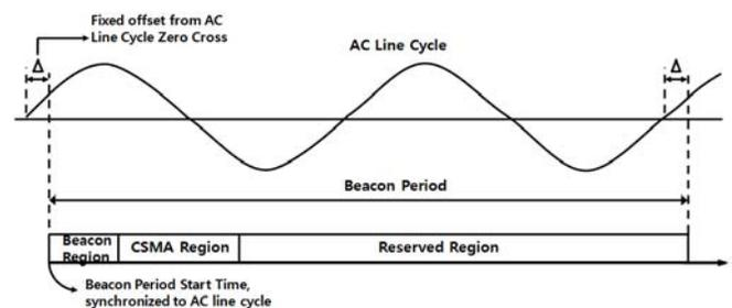
Figure 1. AC cycle synchronization of the Beacon Period
