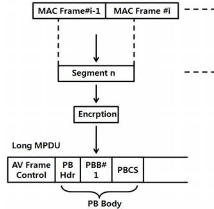
Figure 2. MAC Frame Fragmentation and MPDU Generation
