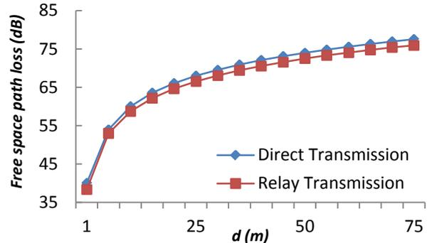
Figure 3. Free space path loss versus distance between source and destination
