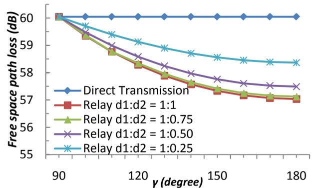
Figure 4. Free space path loss versus  $\gamma$
