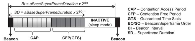
Fig. 1 Superframe structure of IEEE 802.15.4.
