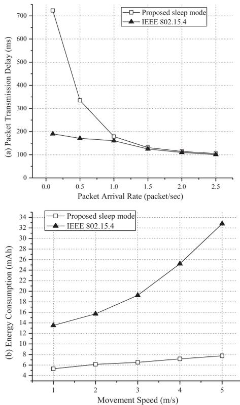
**Fig. 4** (a) Packet transmission delay and (b) energy consumption of the mobile sensor device.
