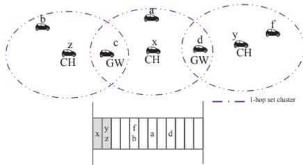
Fig. 11: The reusing time slot in a TDMA frame.
