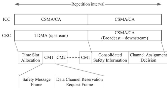
Fig. 2: Time structure in ICC and CRC channels.
