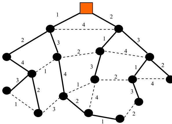
Fig. 2. A Minimum Spanning Tree of a WMN with 4 different channels
