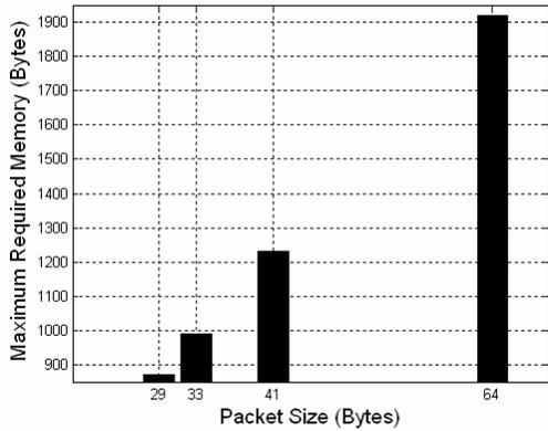
Figure 8. Maximum memory requirements considering different packet sizes.
