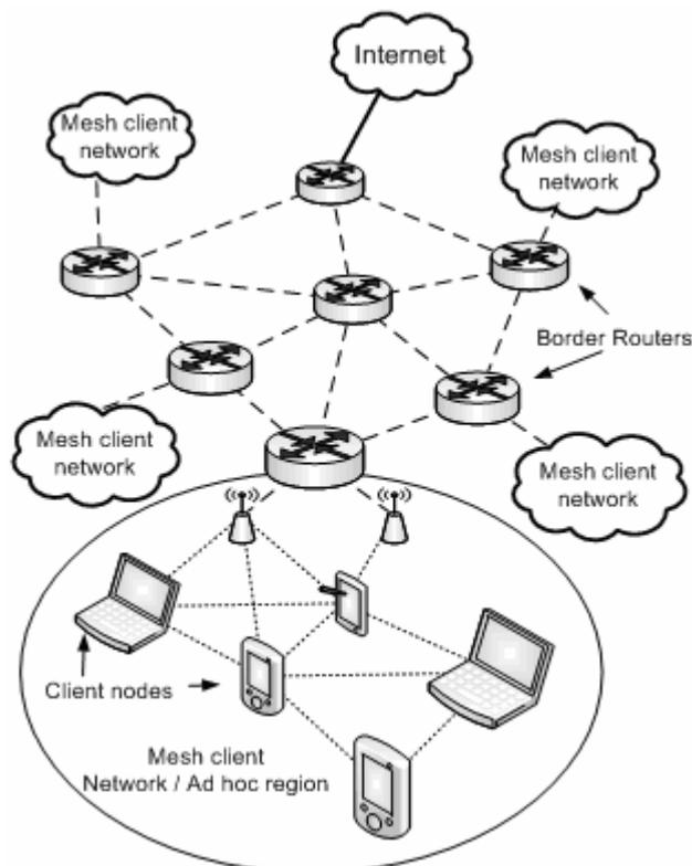
Figure 1. An example of a Hybrid Wireless Mesh Network.
