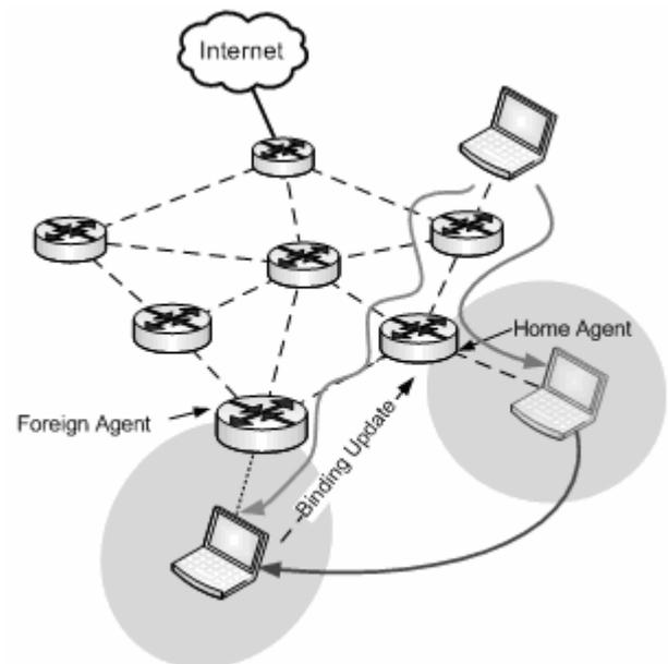
Figure 3. Addressing in Hybrid WMN. Mobile node changing a client mesh network is provided with a care-of-address by foreign agent. Messages to the node are diverted by home agent to the new location.
