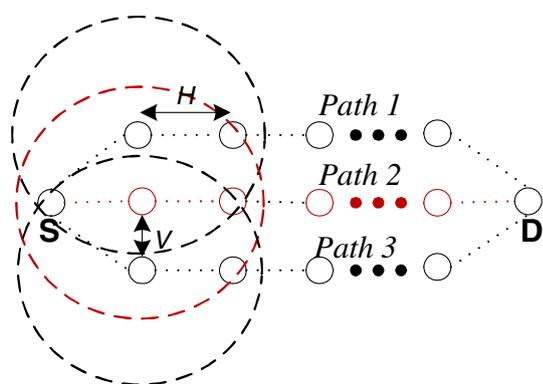
**Fig. 7** Example of grid topology for backbone nodes
