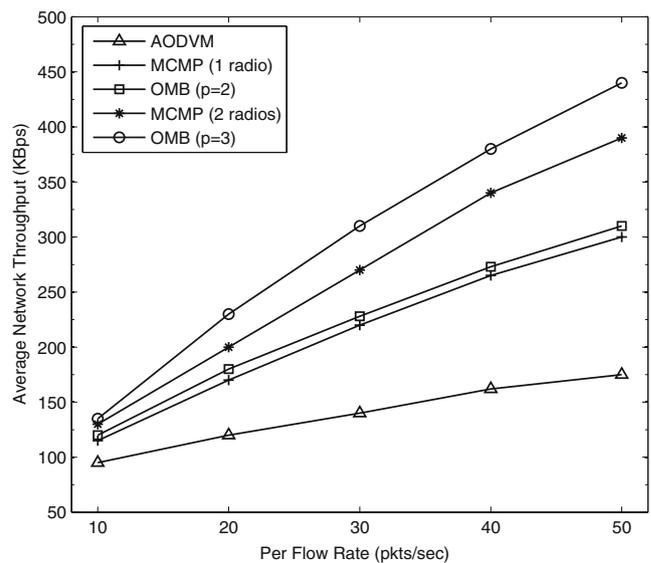
Fig. 15 Impact of traffic load with 15 simultaneous flows
