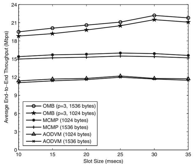
Fig. 10 Impact of slot size
