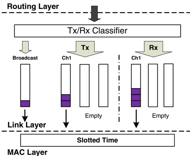
Fig. 6 Queue at nodes communicating on channel 1
