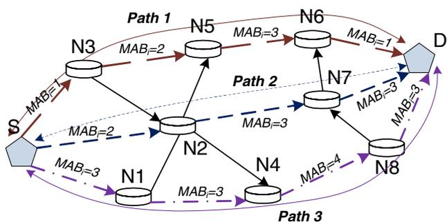
Fig. 1 An example for three node-disjoint paths
