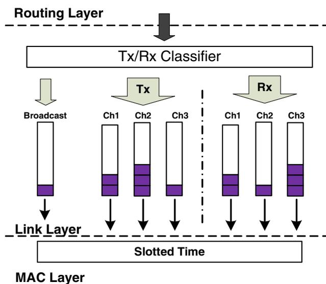
Fig. 5 Queue at two-end backbone nodes
