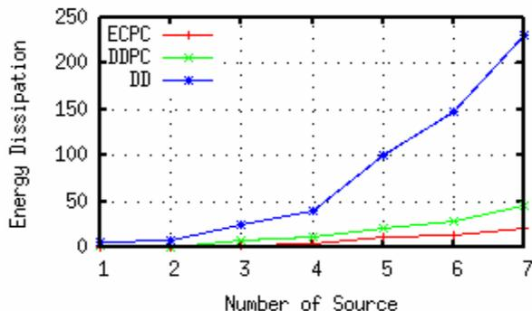
Figure 4. Energy Dissipation for 100 Nodes Placed Randomly into 100X100 Area with Varying Number of Sources from 1 to 7
