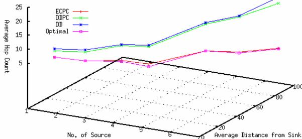
Figure 3. Average Hop Count under Increasing Number of Sources and Average Distance of Sources from the Sink for 100 Nodes Deployed Randomly in a 100X100 Area
