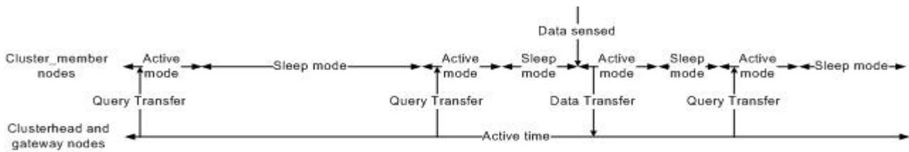
Figure.1. Query Propagation and Data Dissemination between Clusterhead, Gateway and Cluster Member Nodes
