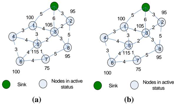
Fig. 1. Sensor network with 8 nodes and each node is labeled with node ID and residual energy and links between nodes are labeled with distance. (a) shows the network before tree construction and (b) is after tree construction
