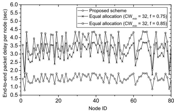
Fig. 6. Source-to-sink delay experienced by packets of nodes in the network.
