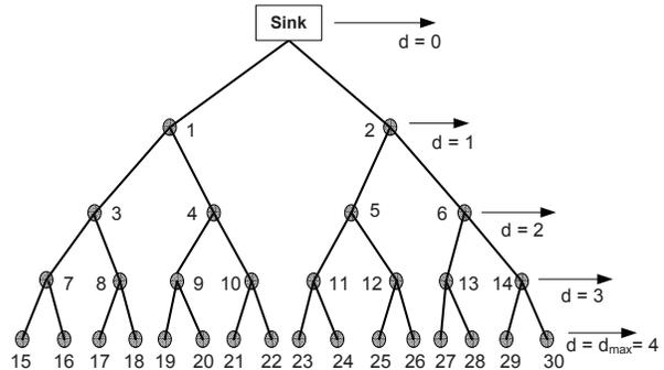
Fig. 1. Network model: a tree topology based wireless sensor network that constitutes a many-to-one data collection paradigm.
