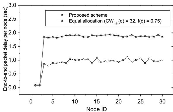
Fig. 3. Source-to-sink delay experienced by packets of nodes in the network.
