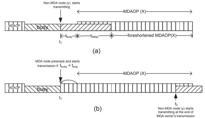
Fig. 3. a. MDAOP of node  $x$  is foreshortened due to an ongoing transmission from non-MDA node  $y$  that starts at  $t_1$ , b. MDA-owner ( $x$ ) preempts and starts its transmission at  $t_1$  before its reserved MDAOP and releases at  $t_2$ .
