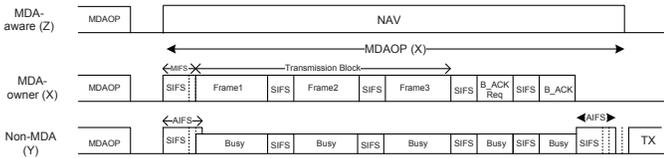
Fig. 2. Proposed access mechanism. MDA-owner node ( $x$ ) starts transmitting after sensing the channel idle for an MIFS period.
