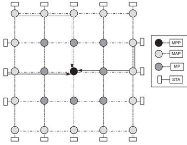
Fig. 4. 25 mesh nodes (16 MAPs, 8 MPs and 1 MPP) are placed in a 5x5 grid. All the STAs transmit voice data to the MPP using 3, 4 or 5-hop routes.
