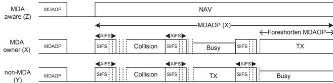
Fig. 1. Node  $X$  can not start at the beginning of its MDAOP due to simultaneous transmission attempt from a non-MDA STA  $Y$ .
