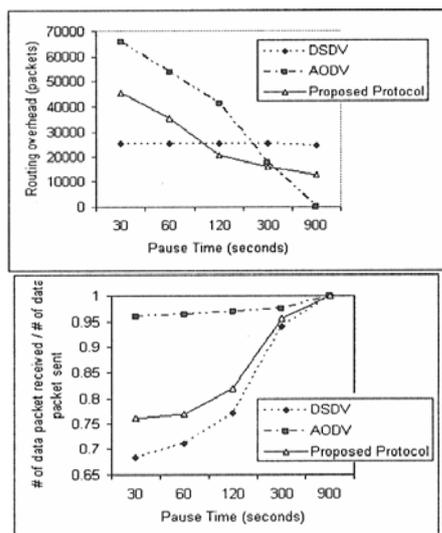
**Figure 4.** (a) Comparison between the 3 protocols of the # of route packet sent as a function of pause time. (b) Comparison between the 3 protocols of the packet delivery ratio as a function of pause time.
