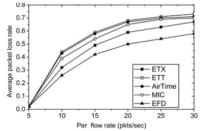
**Figure 5: Average packet loss rate with increasing loads of the active flows.**
