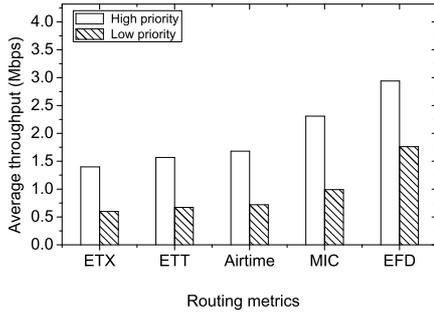
**Figure 6: Average throughput of flows with different traffic priorities.**
