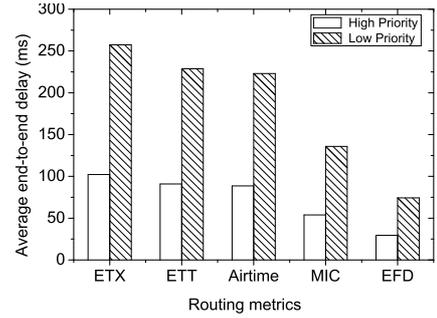
**Figure 7: Average end-to-end delay of flows with different traffic priorities.**
