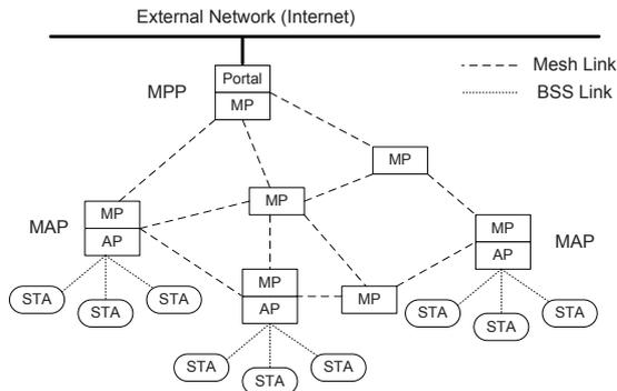
Figure 1: Architecture of an IEEE 802.11s WMN
