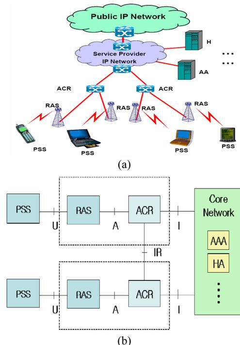
**Fig. 1** Wireless Broadband: (a) Portable Network Architecture. (b) WiBro network reference model. RAS and ACR within the dotted line can be logically integrated as a single entity and is referred to as a wide-sense RAS (fig. source: [2]).
