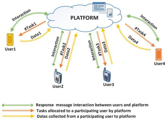
Fig. 1: Crowdsourcing system model with platform-user interaction based incentive mechanism and task allocation
