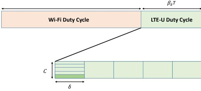
Fig. 2: Duty-cycle distribution among Wi-Fi and LTE-U. LTE-U duty-cycle is further divided into LTE sub-frames for resource allocation to cellular users.
