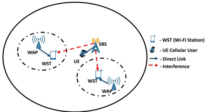
Fig. 1: LTE-U system model. Blue solid lines show the direct communication among the network nodes while the red dotted line shows interference of LTE-U on coexisting Wi-Fi network.
