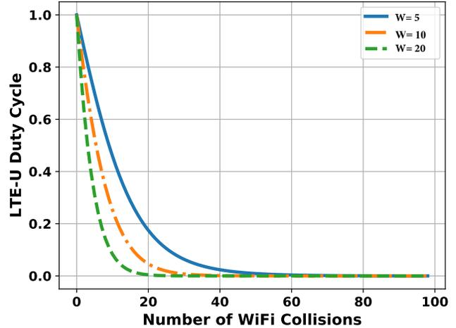
Fig. 4: Plot of Wi-Fi collisions vs. LTE-U duty-cycle
