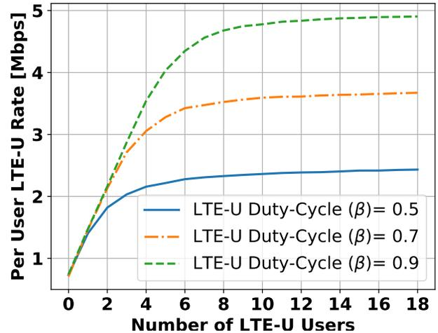
Fig. 5: Plot of number of LTE-U users vs. Per User LTE-U Rate
