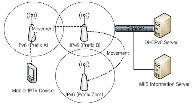
**Fig. 3** Network architecture for handover scenarios using DHCP and IEEE 802.21 Information Server.
