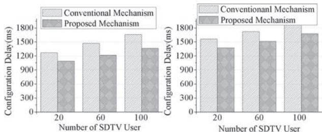
Fig. 4 IPv6 address configuration time delay (left: IPv6 stateless address configuration, right: IPv6 stateful address configuration).
