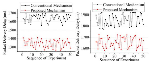
Fig. 5 Packet delay (left: IPv6 stateless address configuration, right: IPv6 stateful address configuration).
