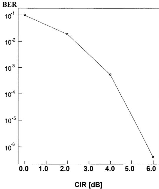
Fig. 3 BER performance only in the colliding part vs. CIR. (Large Packet)
