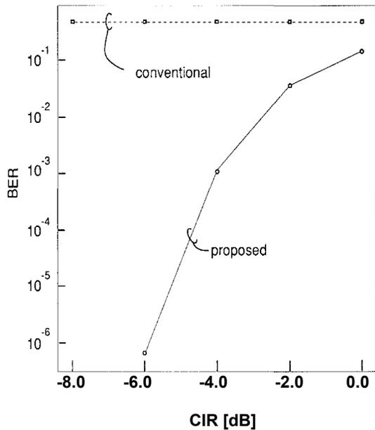
Fig. 4 BER performance only in the colliding part vs. CIR. (Small Packet)
