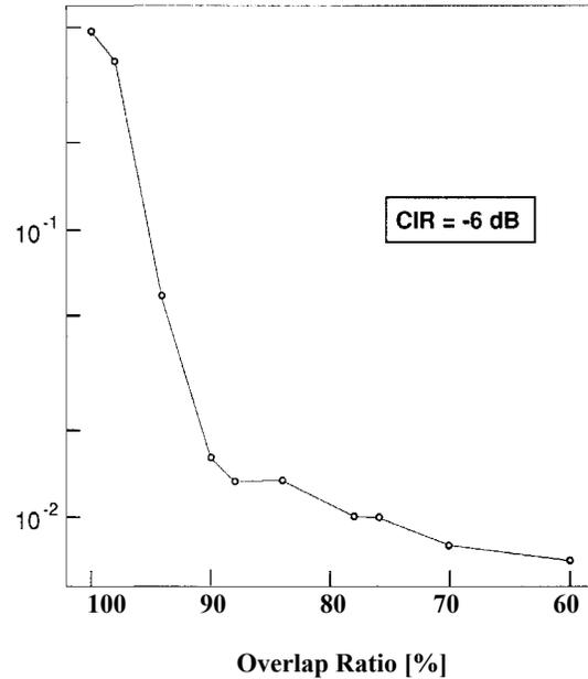
Fig. 5 BER performance vs. Overlap ratio for small Packet
